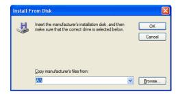
Click on 'Browse...' and then use the standard file window to find the 'USB drivers' folder on the CD. Select 'ftdibus.inf' from this folder and click on 'Open'. The window above will re-appear with a filename at the bottom. Then click 'OK'.
