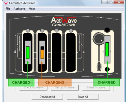
An Actiwave which has been used should be left charging on the reader for a period of several hours, if you require it fully charged. The estimated battery level shown may not be fully accurate during charging itself, so it is advisable to leave the unit connected and charging for some time if the indication has reached green after only a short period.
