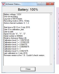
This window provides information about the battery voltage, details of the current device settings, details of the recording and technical information about the Actiwave.
