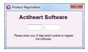
When you register your Actiheart system with CamNtech, you will be supplied with an 8 digit serial number along with the software. This serial number is unique to the user and will enable the user to obtain software support from CamNtech. Once this is done, the software is ready to use.
